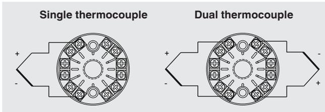
The colour coding at the positive connection to the instruments always decides the correlation of polarity and connection terminal.
