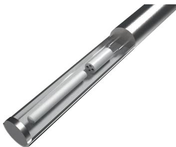
In sheathed resistance thermometers the flexible part of the probe consists of a mineral-insulated metal-sheathed cable (MIMS cable). It features a stainless steel outer sheath, which contains the insulated internal leads, embedded within a high-density ceramic compound. The measuring resistor is connected directly to the internal leads of the sheathed cable.
