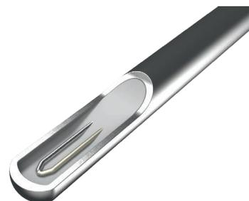
In sheathed thermocouples the flexible part of the probe consists of a mineral-insulated metal-sheathed cable (MIMS cable). It features a metal outer sheath, which contains the insulated internal leads, embedded within a high-density ceramic compound. Sheathed thermocouples, due to their flexibility and the small diameters that are possible, can be used in areas that are difficult to access.
